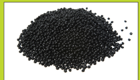
Recycled Post Consumer Carpet material is available as PC4 - Post Consumer Carpet Calcium Carbonate - as well as fiber and pellets.
